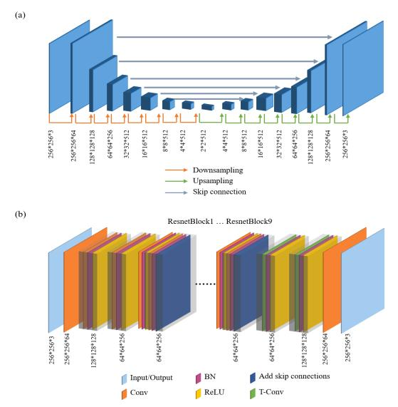
**Fig. S1.** Schematic diagram of the structure of generators in U-FBNet and R-FBNet. The generator in U-FBNet. (b) The generator in R-FBNet.
